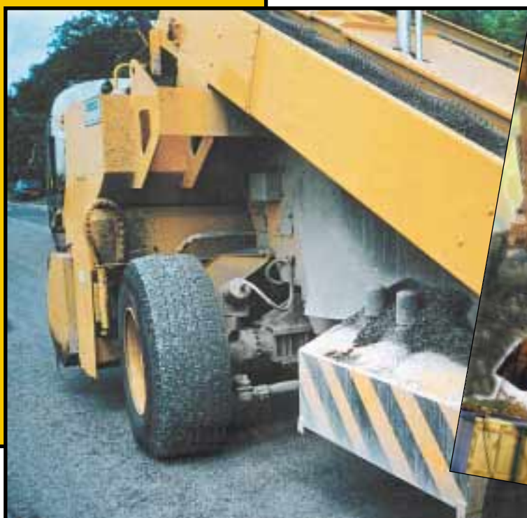
This chipper spreader reversed over a worker, who lost his leg in the accident
